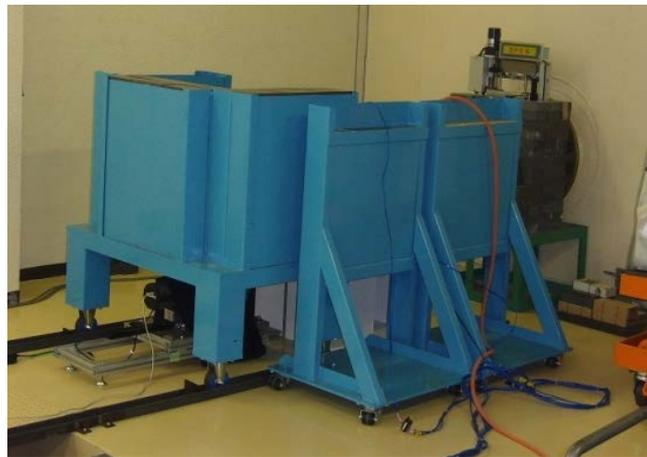
Fig. 2 Radiation shielding in B4 port
