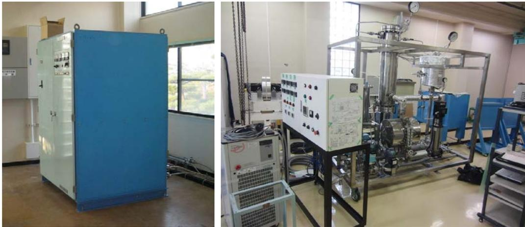
Fig. 1 High power supply system(left) and water loop (right) for two phase flow research using neutron radiography in B4 port
