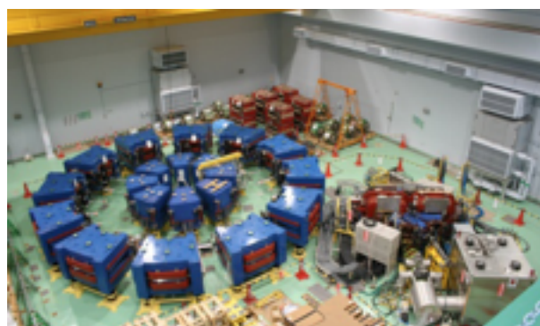
Fig. 3. FFAG complex at KURRI for ADSR experiment [18,19,20].
