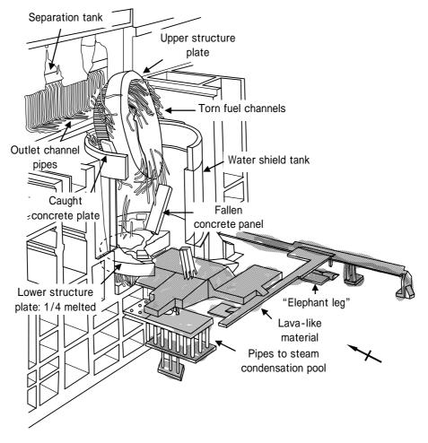
Fig. 14. Cross sectional view of the destroyed reactor.
