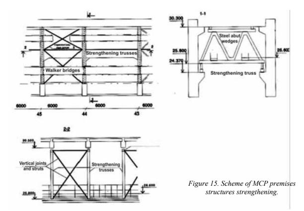
and requires the urgent strengthening. Couplings of ferroconcrete girders with the columns along the row  $\Gamma$  and ferroconcrete wall near row E are partially destroyed, the girders are displaced from supporting cantilevers.
