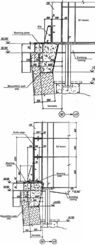
Figure 17. Strengthening of E1 beams supporting parts and ferroconcrete wall along axis 50 in place of resting upon it of E1 beams unit (row *H*)
