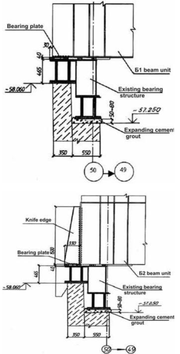
Figure 19. Strengthening of B1 beams supporting parts and metallic support under B1 beams in place of B1 beams unit abutting on ferroconcrete wall along axis 50 (row  $\Pi$ )
