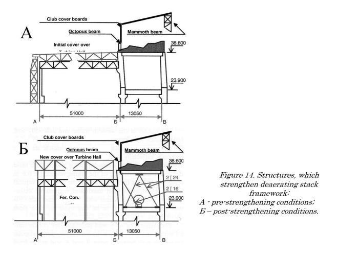
Besides, in 1988, trusses of turbine hall coating were dismantled, which were resting upon the cantilevers of row *B* columns (design decision of 1986), and instead of them the new coating was assembled with resting upon steel-concrete walls, newly erected in turbine hall between the rows A-*B* along axes 41 and 49.
