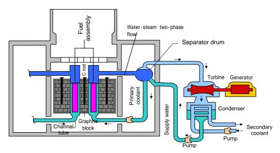
Fig. 2: Basic scheme of RBMK
