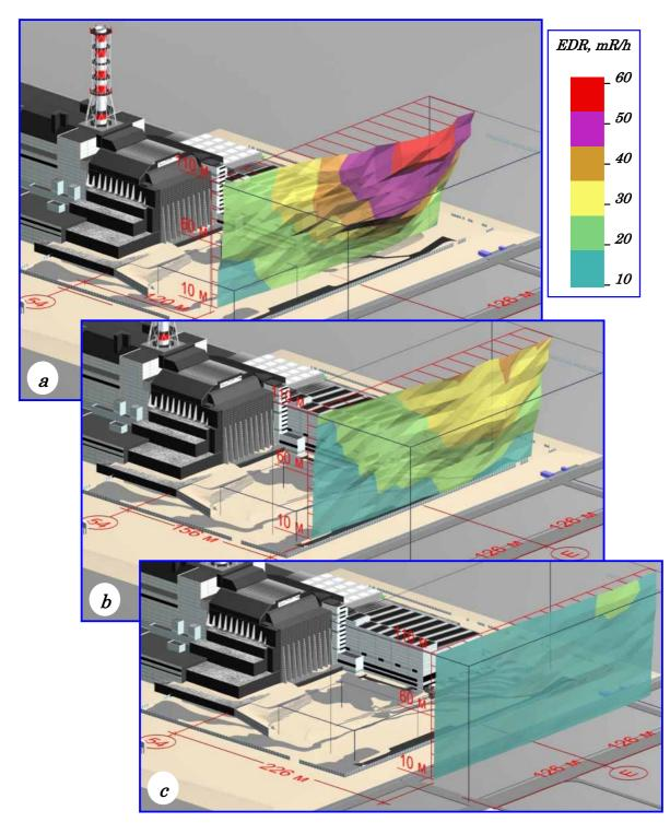
Figure 13 – Model of gamma-field in NSC erection zone (June 2004) a – cross-section along axis 54 + 120 m;
