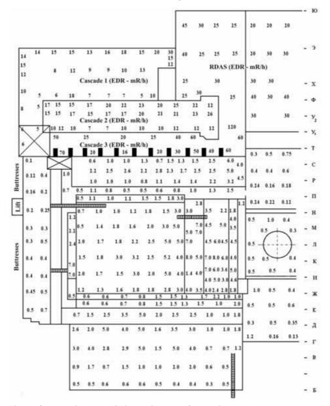
Figure 11 - Chart of EDR value on «Shelter» object roofing in the axes 35 - 54, rows B - HO
