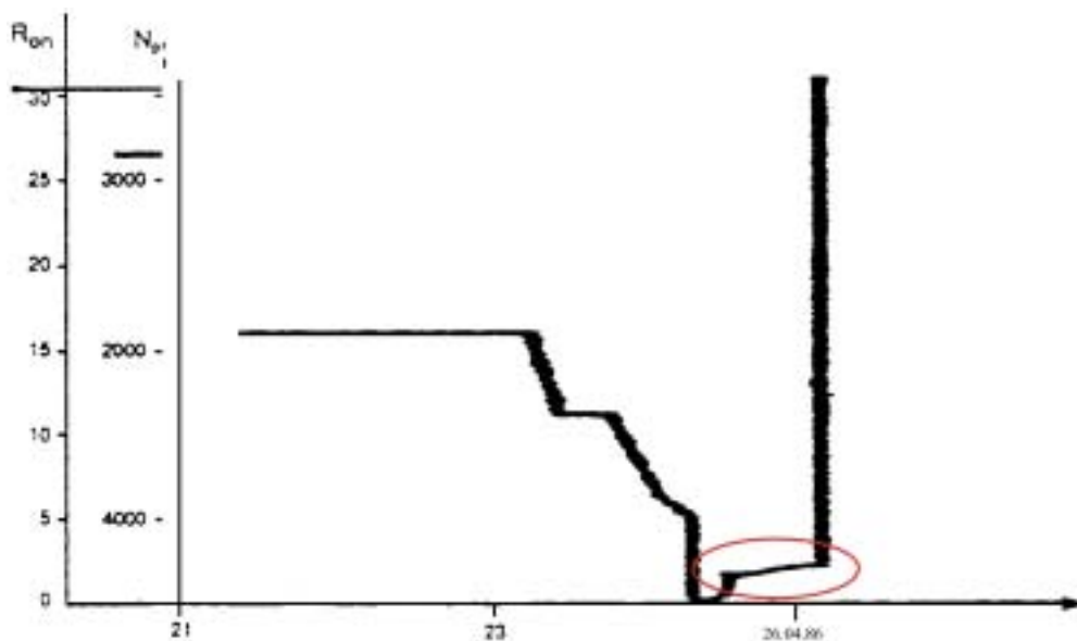
Fig.2. The change of the power ( N_p ) of the Unit-4 reactor in the diapason of the time from 23 h 00 min 25.04.1986 to the official moment of the accident 26.04.1986 .(The magnified part of the curve in Fig. 1). The unabated increasing of the reactor power calls attention.
