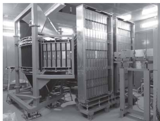
Fig. 8. Special environment neutron powder diffractometer, SPICA, installed at the BL09 beam port in J-PARC/MLF [6].
