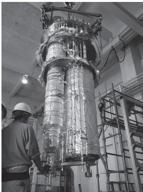
Fig. 3 Photograph during a cryogenic test of the helium cryostat, one of the critical components of the TUCAN UCN source. Adapted from Ref. [18].
