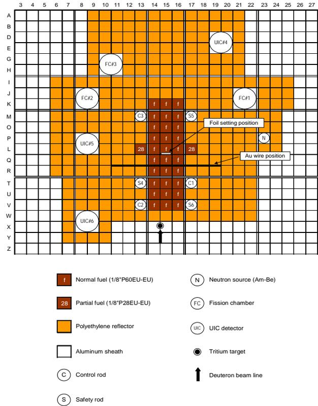
Fig. 1. Top view of A-core configuration.
