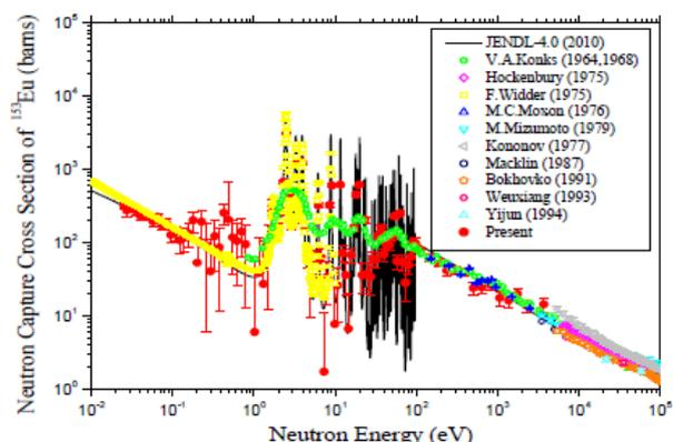
Fig. 2. Neutron capture cross sections of  $^{153}\text{Eu}$
