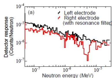
Fig. 3. Response function of the prototype detector measured with and without the silver filter.
