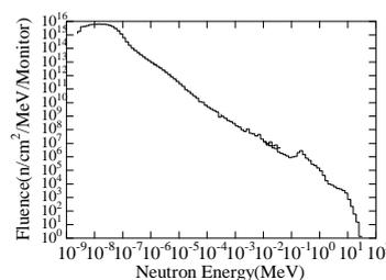
Fig. 2. White neutron spectrum at KURRI measured with the <sup>6</sup>Li-glass scintillation detector, the NE213 liquid scintillation detector and the total absorption BGO detector.
