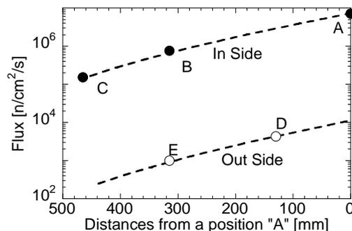
Fig. 2. Results of flux measurements in our measurement condition. Notations of “A” to “E” are represented in Fig.1 (b).
