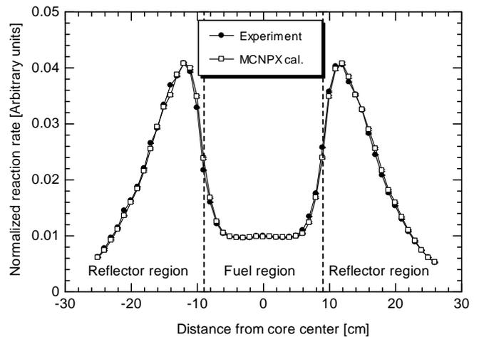
Fig. 2. Comparison between the results in experiments and calculations (MCNPX) of Au reaction rates.
