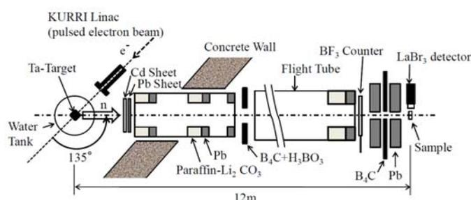
Fig. 1. Experimental set-up at linac of KURRI.
