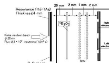
Fig. 1. Schematic view of the prototype of epithermal neutron camera and the experimental setup at KURRI.
