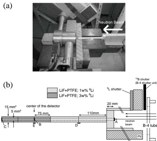
Fig. 1. (a) A photograph of our experiment at the B-4 experimental room. (b) A schematic drawing of a developed collimator. Positions of “A” to “E” are used to measure neutron fluxes in the beam axis, and those of “D” and “E” are used to evaluate the leakage ones.
