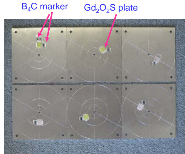
Fig. 1 Gd plates and B 4 C marker for Dy foil transfer method
