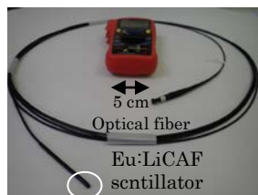
Fig. 1 Detector coupled with the optical fiber.
