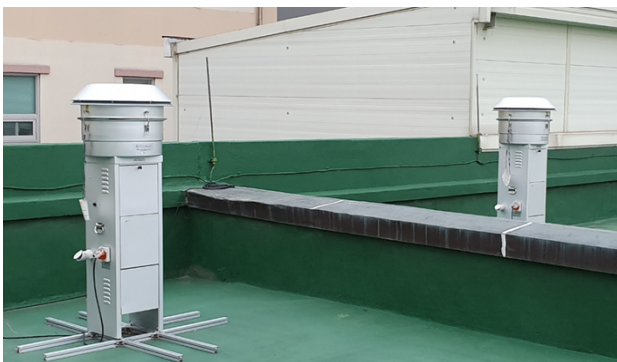
Fig. 1. A photo of PM10 and PM2.5 samplers in Daejeon.
