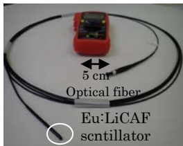
Fig. 1 Detector coupled with the optical fiber.
