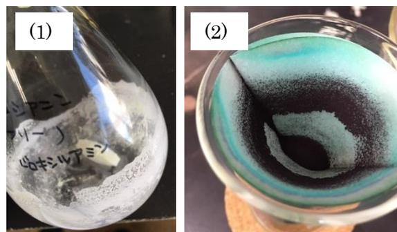
**Figure 2 Pictures of synthesized chemicals, (1) metal free Pc and (2)Pc-Zn**
