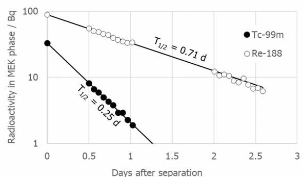
Fig. 2. Radioactive decay curve of  $^{99\text{m}}\text{Tc}$  and  $^{188}\text{Re}$
