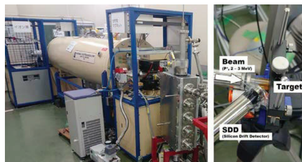
Fig. 2. In-air PIXE analysis system at TCU-Tandem.
