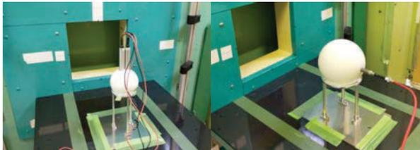
Fig. 1. BSS with a pair of lithium-glass scintillators (left) and BSS with a <sup>6</sup>LiF-shielded <sup>3</sup>He proportional counter (right).
