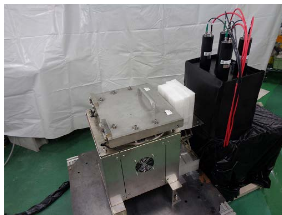
Fig. 1. The rotation machine (left), the water Cherenkov detector (right), and measurement object containing HEU (middle).
