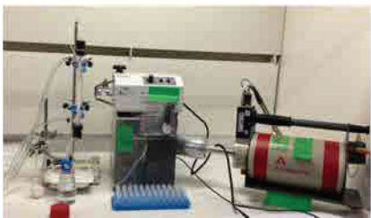
Fig.1. Extraction-chromatography set-up with on-line γ-ray detector for Yb/Lu separation.
