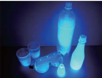
Fig.1 Scintillation light from plastic materials with excitation by UV light and ionizing radiation.
