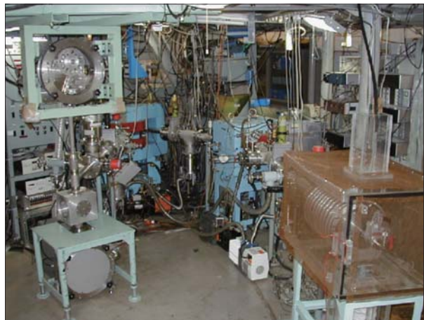
The nuclear beam facility with two beam lines; nuclear study course with a tape collector (left side) and material study course with a post accelerator (right side).
