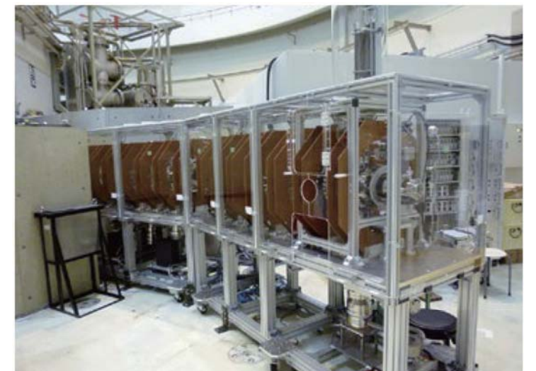
Reactor-based slow positron beam system at the KUR B1 hole.
