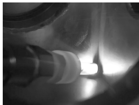
Fig. 3. Sample and quartz container during laser irradiation.
