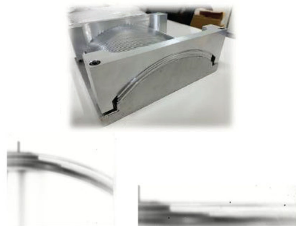
Fig. 9. Stator coil structure and visualized coolant profile. (a)Snapshot, (b) Converted to cylindrical coordinate.
