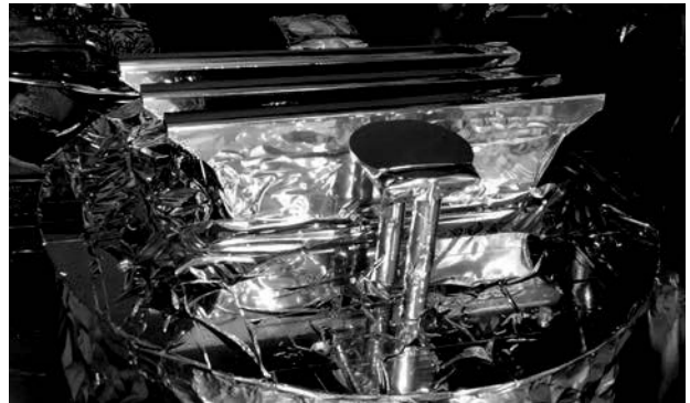
Fig.1 Photograph of three parts of ellipsoidal neutron supermirrors coated by the ion beam sputtering instrument (KUR-IBS) at KURNS.
